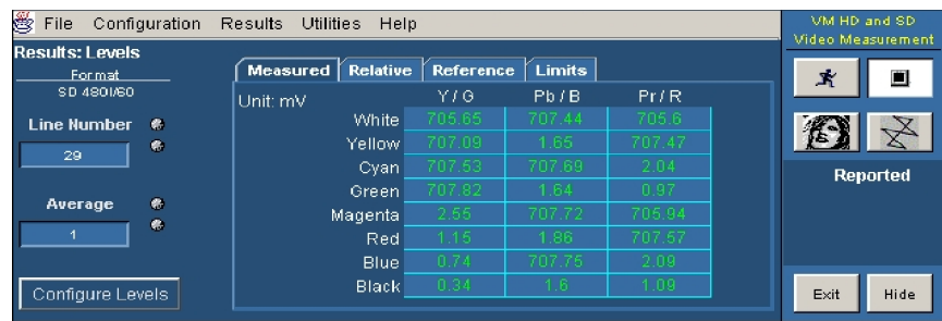
Figure 3-36: Displaying the Levels measurement
