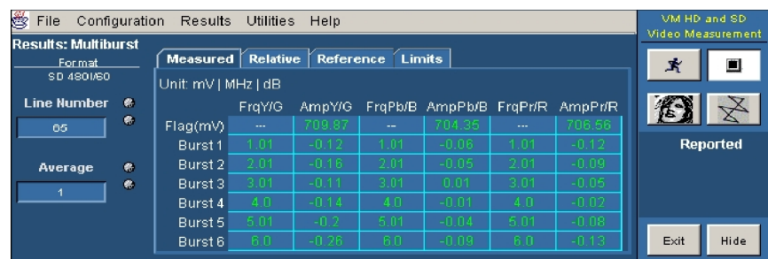
Figure 3-38: Displaying the Multiburst measurement
